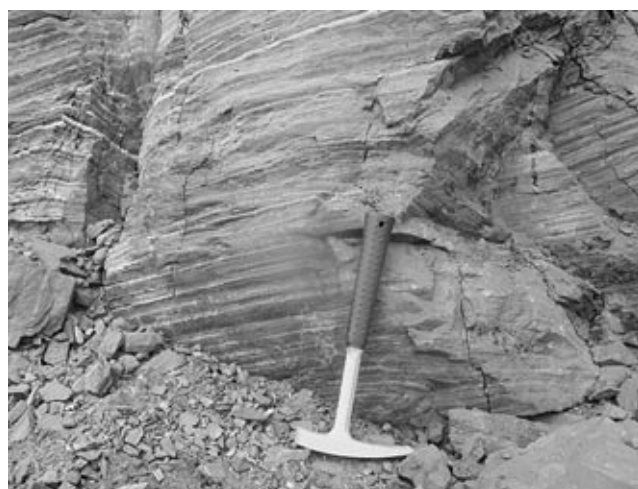
Fig. 3. BIF with alkaline amphiboles, sampling site L-5, Lebedinskii opencast mine, northern wall, level –110 m. Dark gray layers consist of quartz and magnetite, pale gray layers are made up of ferriwinchite and aegirine-augite, very pale layers are composed of calcite and dolomite.
